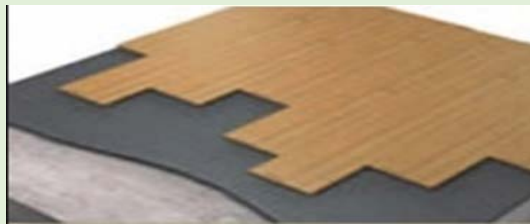
Concrete → Mat → Floor Tiles → Mat → Floor
