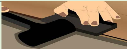
A tapping hammer and block
