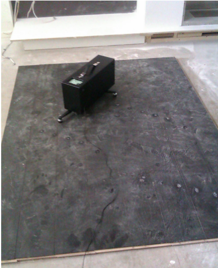
Figure 1: Tapping machine in-situ
