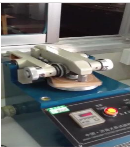
ROTARY SANDER TESTING WEAR LAYER
