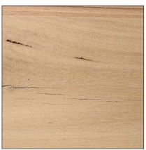
Checks are a separation of the wood fibre and differ from a split in that they do not travel from one surface of a board to another. They can often occur with rapid drying and be over much of the board surface. However, grain
